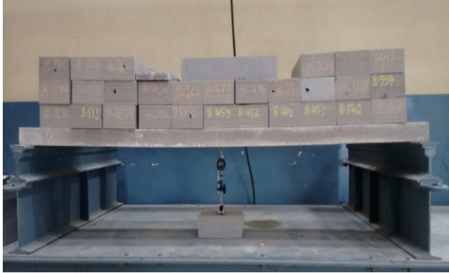
Fig. 7.1: Ultimate load arrangement on wall panel
